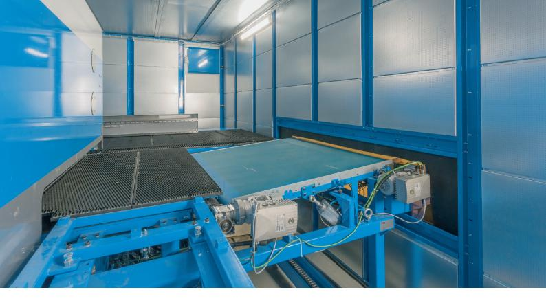
With an effective enslosure around a noisy machine, the working conditions and occupational safety of staff are improved and floor space near the machine is freed up for other uses.
